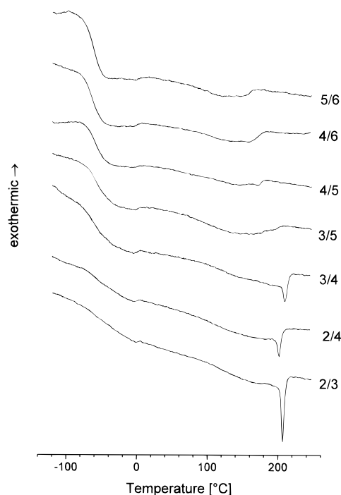
Figure 5. DSC scans of PPP(EO) x/y with different side-chain lengths, normalized to the same sample mass.
